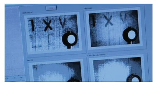
Example imagles of blood stains captured using the prototype IR camera that was developed with the support of NIJ funding.
