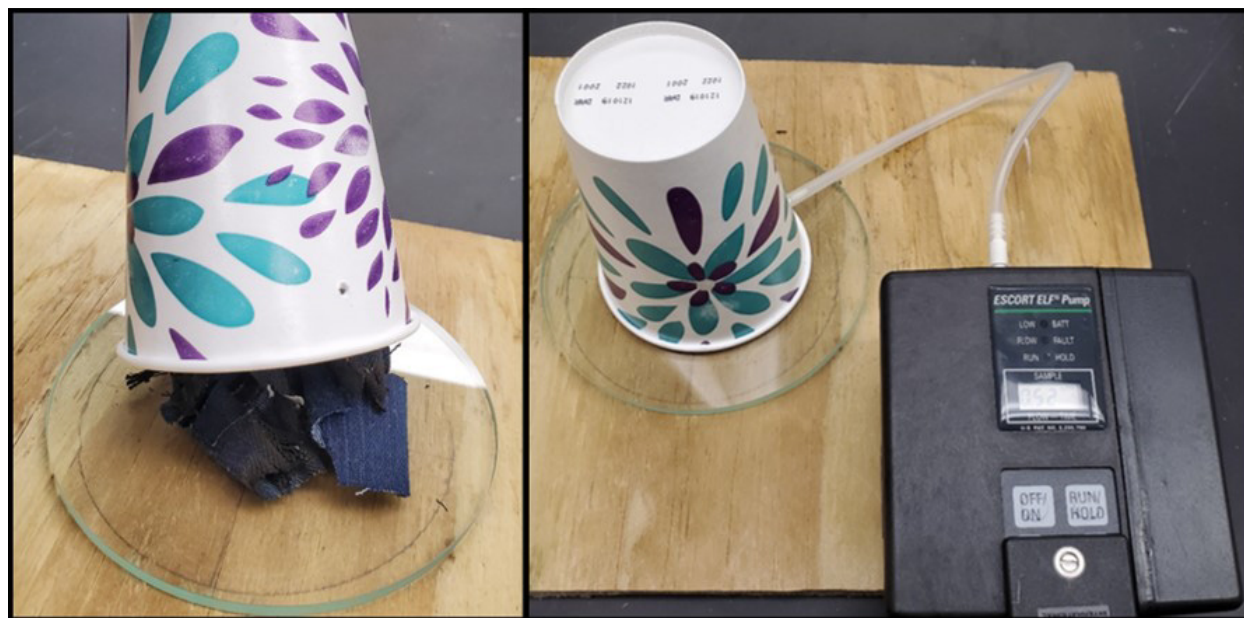
Figure 1: Photograph depiction of the CMV/Cup apparatus with debris placed on the glass platform (left) and the CMV sampling using the hand-held vacuum pump (right).
