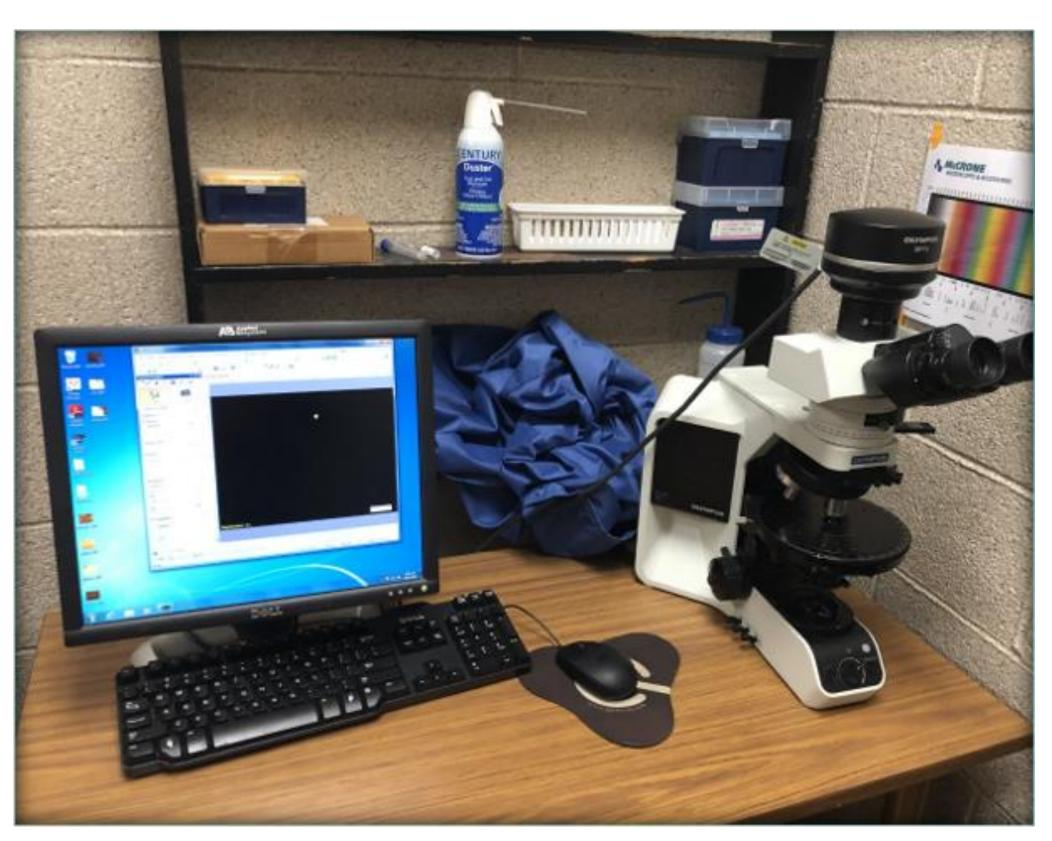
**Figure 2 – Olympus BX53 Polarized Light Microscope**
