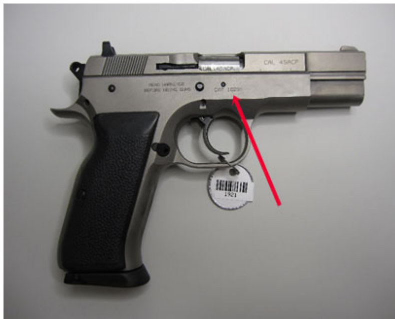
Figure 1. Tanfoglio Witness pistol with dot pin-applied, and grinding and sanding removed, serial number.
