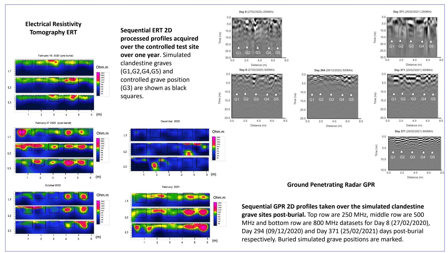
Figure 3. Geophysical Techniques Profiles
