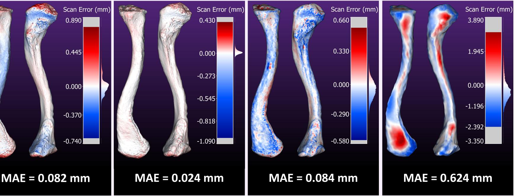
Figure 4. Examples of scan error heat maps for three examples (femur, scapula, clavicle) of the eight selected bones. Error is relative to the reference scanner (mm). Heat maps are accompanied by the grand MAE value (mm) for that scanner.
