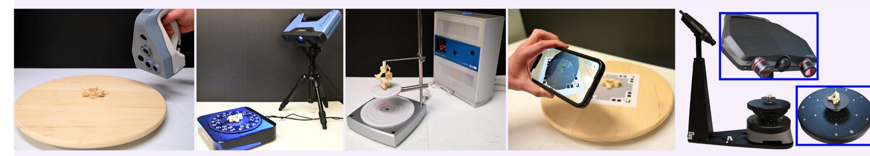
Figure 2. 3D scanners used. From left to right: Artec® Spider® (\$17.5K), EinScan® Pro 2X (\$6K), NextEngine® Ultra HD (\$3K), Qlone® photogrammetry (\$0), Solutionix® C500 (\$38K).
