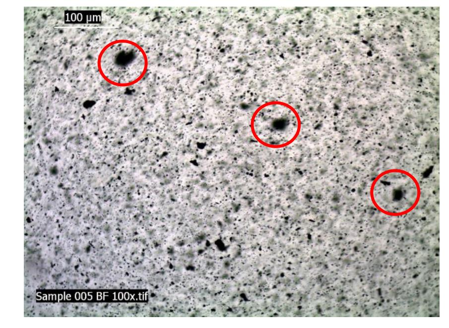
Figure 1. Microphotograph of grease sample. Red circles indicate the observed particles that were part of the original manufacturing formulation
